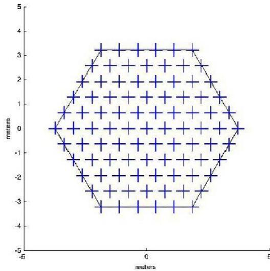
Figure 2. Antenna elements in the Sub-array.
