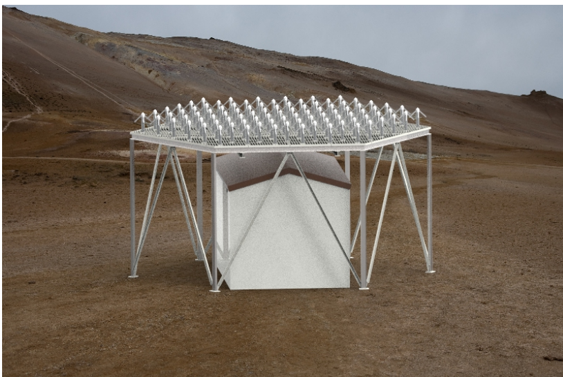
Illustration of arrangement of antenna elements in one hexagon.* @EISCAT Scientific Association
